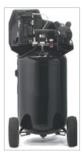
Cast iron, twin cylinder, oil lubricated pump features one-piece cast iron crankcase, thermally stable cast iron cylinder body, aluminum head and machined cast iron valve plates, automotive style ball bearings, durable stainless steel reed valves, oil level sight glass, easily accessible oil fill, 12" cast iron balanced flywheel
